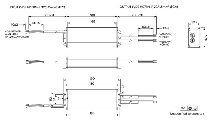
**Note:** The 2 DC output cables are connected in parallel internally because one 1.5mm<sup>2</sup> wire can only carry 14.5A. Please connectthe 2 brown wires together and 2 blue wires together in application, or ensure each cable carries same current.
